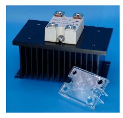
Heat Sink Dimensions: 5.25" x 3.0" x 2.75" Overall size w/Single SSR and Touch Safe Cover & DIN Clip: 5.25" x 3.0" x 4.25" Anacon's "Cool One" heat sink designs provide a thermally optimized Panel mounting platform for today's high performance solid state relays. The listings below provide the actual load currents that each part type will support. If you're not sure about how to select the correct product for your application, call Anacon, toll free and discuss your application with us.
